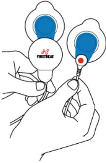
1. Attach the electrodes to the cable and device end.
