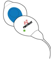
4. The measurement starts automatically when the device is attached. Make sure the green led is flashing. Note: The light is easiest to see in a dark room.
