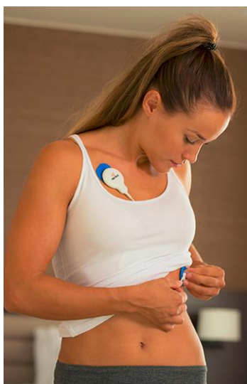
Figure 3. The Bodyguard 2 measurement device is an easy-to-use R-R interval recording device designed for the Lifestyle Assessment measurements.
